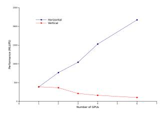
Splitting the lattice along the minor dimension leads to sub-domains composed of non contiguous memory cells, which has dramatic effects on performance.
