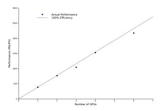
We measured up to 2.17 GLUPS (94% efficiency) using 6 Tesla C1060 on a  $192^3$  lattice in single precision.
