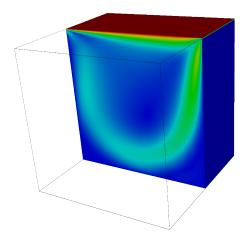
To validate our code, we implemented the lid-driven cubic cavity test case. The lattice is split in cuboid sub-domains along the major dimension.
