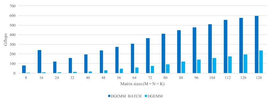
Configuration Info - Versions: Intel® Math Kernel Library (Intel® MKL) 11.33; Hardware: Intel® Xeon® Processor E5-2699v3, 2 Eighteen-core CPUs (45MB LLC, 2.3GHz), 64GB of RAM; Operating System: CentOS 7.1 x86 64
