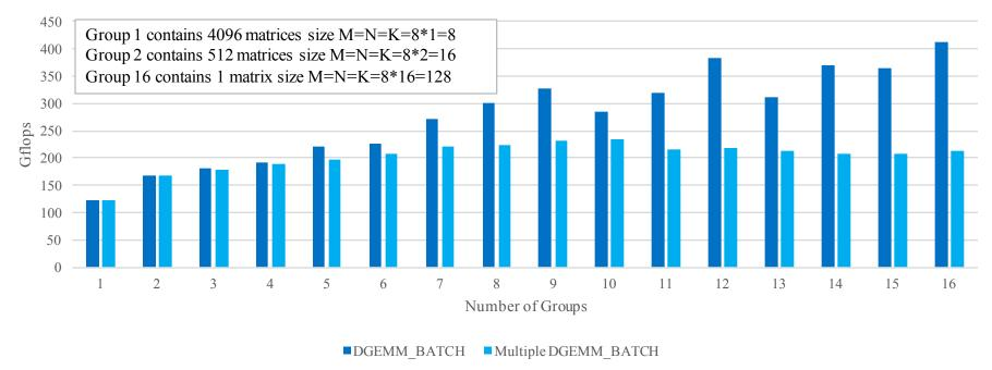
$Configuration\ Info\ - Versions.\ Intel @\ Math\ Kernel\ Library\ (Intel @\ MKL)\ 11.3\ 3; Hardware:\ Intel @\ Xeon @\ Processor\ E5-2699v3\ , 2\ Eighten-core\ CPUs\ (45MB\ LLC\ , 2.3GHz)\ , 64GB\ of\ RAM;\ Operating\ System:\ CentOS\ 7.1\ x86\_64B\ of\ RAM;\ Operating\ System:\ Operating$
