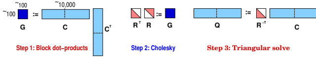
Figure 4: Illustration of CholQR on two GPUs, where the dashed lines show the matrix distribution.
