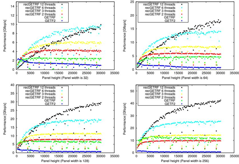
**Fig. 5.** Scalability study of the recursive parallel panel factorization in double precision on LAPACK layout with various panel widths: 32 (top-left), 64 (top-right), 128 (bottom-left), and 256 (bottom-right).
