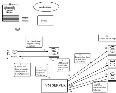
**Fig. 2.** Event sequence for a distributed plug-in loading
