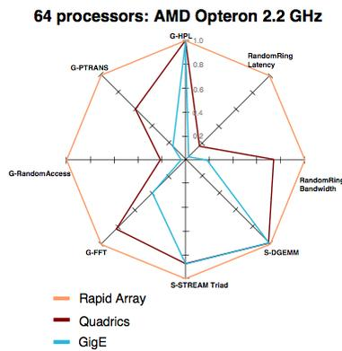
Figure 5. Sample kiviati diagram of results for three different interconnects that connect the same processors.
