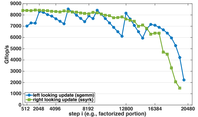
Figure 7: The performance of the gemm and syrk routine for the shape required by the update of either the left or right looking design when varying the size of nb in both single and double precision on a Nvidia P100 GPU.
