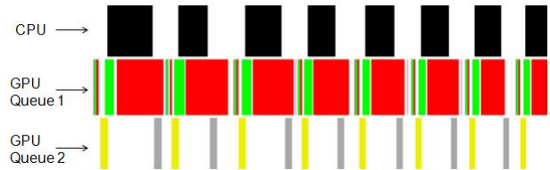
Figure 7: Partial CPU-GPU execution trace of a hybrid LU factorization in cMAGMA based on the two command-queues’ optimization, overlapping CPU-GPU data transfers (the yellow and gray transfers in GPU Queue 2) with GPU work (in GPU Queue 1).
