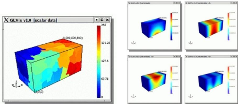
**Fig. 2.** Our eigen-solver's library applied within **ParaGrid**. Left: partitioning of the computational domain into 256; Right: the 4 lowest eigenmodes for an elasticity problem (solved in parallel on 256 processors).
