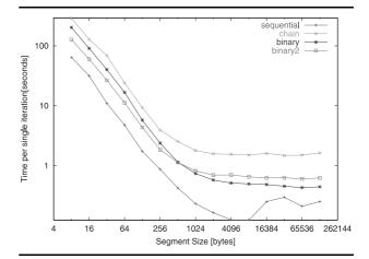
Fig. 2 Segment size versus time for various communication methods.
