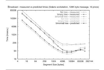
Fig. 10 Comparison of algorithms: measured versus predicted times.
