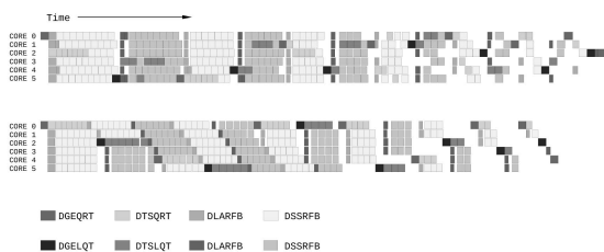
Fig. 3. Scheduler tracing with six Intel Tigerton 2.4 GHz cores: top dynamic—bottom static.
