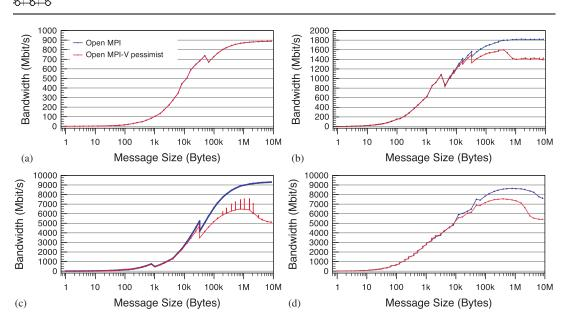
Figure 5. Ping-pong performance comparison between Open MPI and Open MPI-V pessimist on various networks: (a) TCP Gigabit Ethernet; (b) MX Myrinet 2G; (c) MX Myrinet 10G; and (d) Shared Memory.
