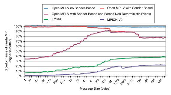
Figure 4. Myrinet 2000 ping-pong performance of pessimistic message logging in percentage of non-fault-tolerant MPI library.
