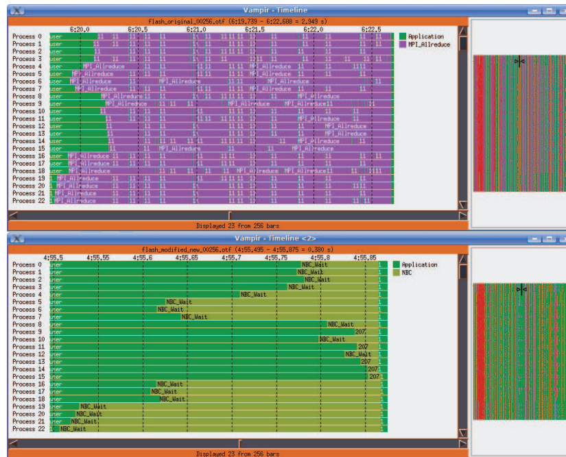
Figure 2: Corresponding communication patterns of MPI_Allreduce in the original code (top) and NBC_Iallreduce plus NBC_Wait in the optimized version (bottom). The latter is more than seven times faster.
