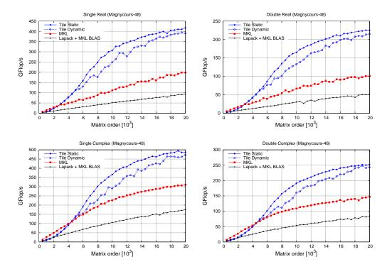
Fig. 6. Performance of SRBT-LDL<sup>T</sup> against MKL and LAPACK.
