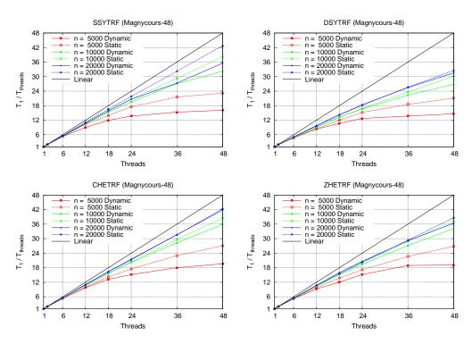
Fig. 8. xSYTRF/xHETRF scalability; dynamic (solid line) and static (dashed line) scheduling.
