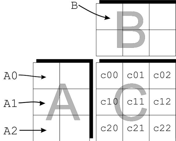
Figure 3:  $M_0 = 3$ ,  $K_0 = 2$ ,  $N_0 = 3$  register-blocked matrix multiply diagram.
