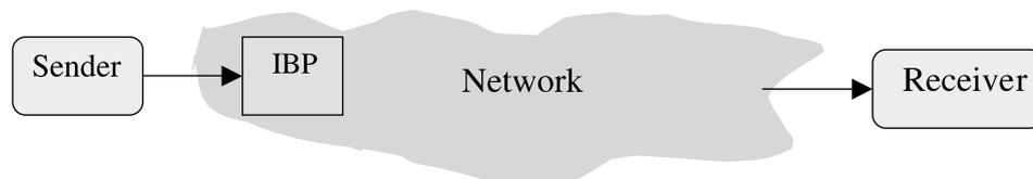
Fig. 1. IBP: keeping data close to sender.
