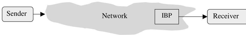
Fig. 2. IBP: place data close to receiver.
