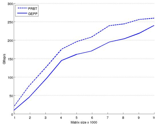
**Fig. 3.** Performance for PRBT and GEPP in double precision arithmetic ( $4 \times 12$ -Core AMD Opteron 6172 @ 2.1 GHz - GPU Fermi Tesla S2050 @ 1.15 GHz).
