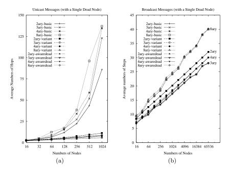
Fig. 2. Message transmission during failure situations. (a) Unicast (b) Broadcast
