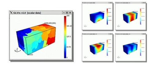
Fig. 2. Our eigen-solver's library applied within ParaGrid. Left: partitioning of the computational domain into 256; Right: the 4 lowest eigenmodes for an elasticity problem (solved in parallel on 256 processors).
