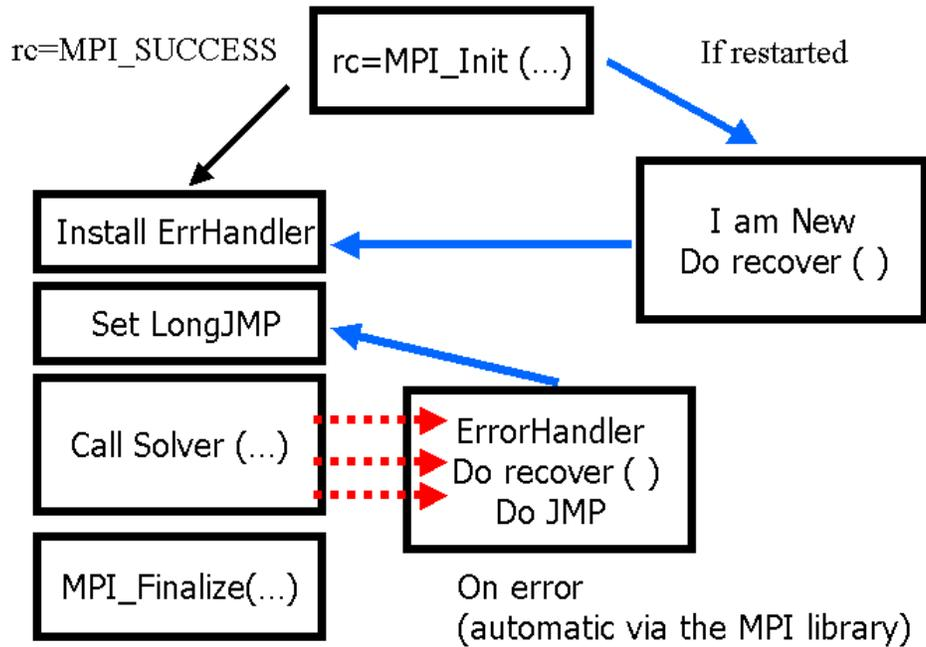
**Figure 1.** Flow control in a typical FT-MPI application using MPI Error Handlers.
