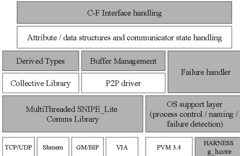
**Figure 2.** Overall structure of the FT-MPI implementation.
